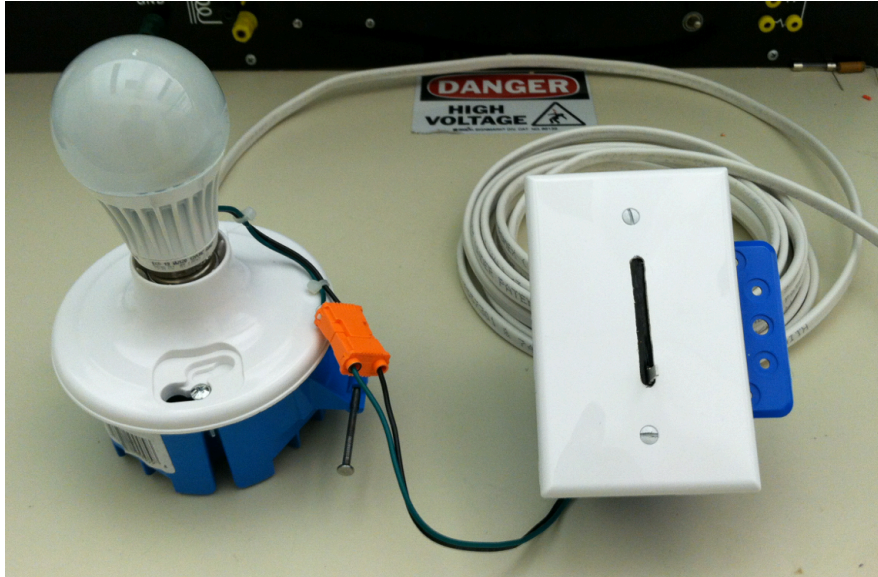
Figure 5-28: A19 DC Light Bulb (left) With Dimmer Box (right) – Fully Assembled.
