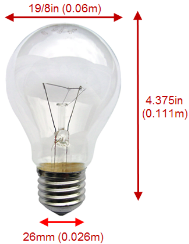
Figure 3-1: Standard A19 Light Bulb and E26 Screw Base Dimensions.
